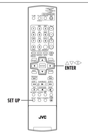
Various modes of this unit are categorized into menus nested in 2 levels shown in the following table. To change the settings of these modes, find the desired mode in the menu (for details on each menu, see pages 93 through 96), then follow the procedure below.
